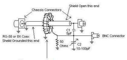
T1 = 10 turns on F-32-43 Toroidal Core
